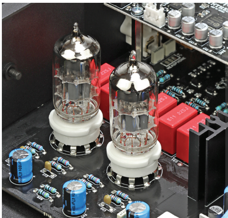
The ECC88 double triode output valves, used as cathode followers to act as low output impedance line drivers. They also impart the 'valve sound', bringing air and space to the sound stage.
